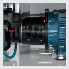
The direct drive connects the air end via coupling to the motor.
