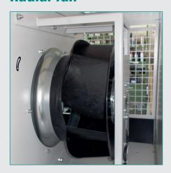
RS-PRO D range compressors are cooled by radial fans. These ensure excellent residual thrust and a pleasant noise level.
